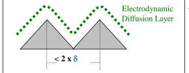
← Microprofile: Diffusion layer thickness surface roughness. Mass transport control results in a non-uniform current distribution.
