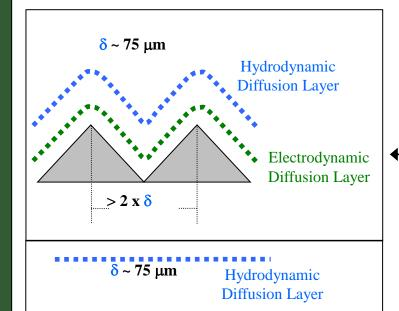
The appropriate waveform can alter the thickness of the pulsating diffusion layer and effectively focus or defocus the current distribution to create non-uniform or uniform deposition respectively.
