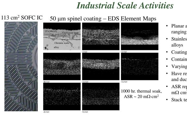
Planar and patterned interconnects ranging from  $100 - 225 \text{ cm}^2$ Stainless steel alloy & proprietary Coatings from a few microns to 50 µm Contained proprietary flow fields • Varying ratios of Co:Mn Have received reports of good adhesion and ductility for the oxide coatings • ASR reported in the range of 10 - 20 $m\Omega \ cm^2$ • Stack testing next
